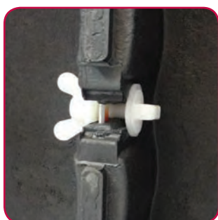
Single nylon fixing secures panel to base (view from underneath)
